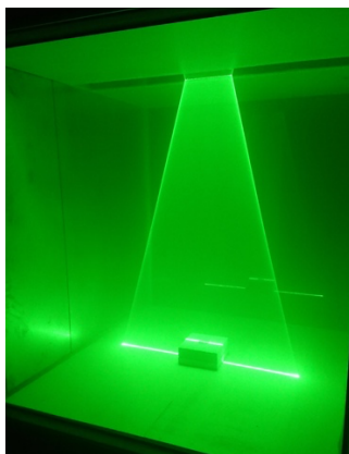
Fig 1. Visualization of the plume using laser techniques
